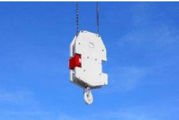
The connectible HiSPS assistance system operates using battery-powered sensors on the trolley and hook block of the crane hook. Connected to a control unit in the switch cabinet, it detects the rope's movements and automatically adjusts the motion and speed of the slewing gear and trolley to it.
