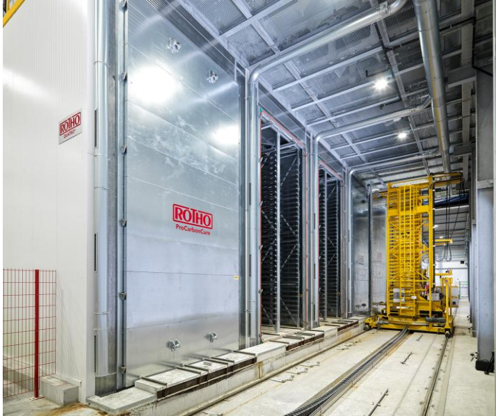
Front of the ProCarbonCure --system for CO 2 -negative facing bricks
